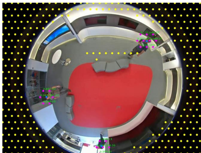
Figure 1. Example of detection results in an omnidirectional image. Purple dots represent the activated classifiers, blue dots represent the final person location. Yellow dots correspond to untrained classifiers.
