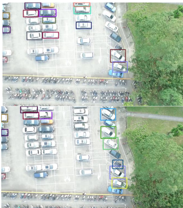
Figure 23 IOU-tracker on the CARPK dataset with ground-truth as the detections. Because of low FPS of video footage, fragmentation and the number ID-switches are very high, therefore this tracker is not applicable to such datasets.
